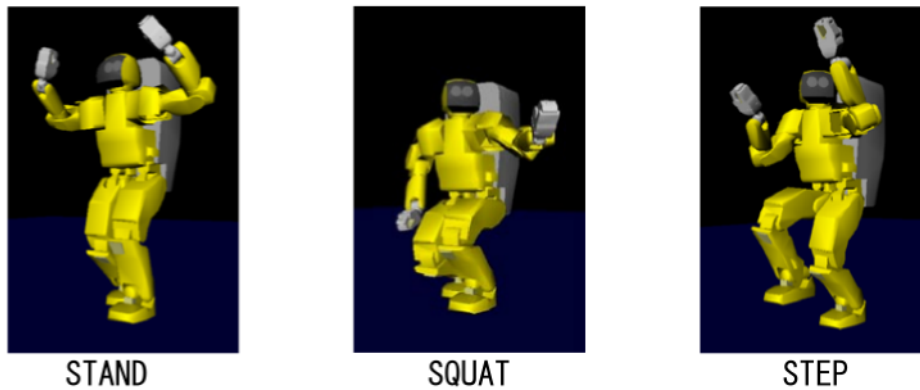
Figure 2.7: Leg motion primitives for dancing. Adapted from [24].
