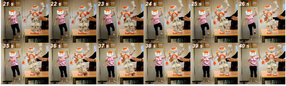
Figure 6.13: Moments during support transition, here showing DS-RS-DS .
