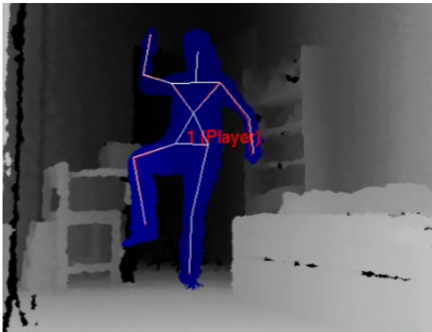
Figure 5.4: Skeleton tracking with NiTE .
