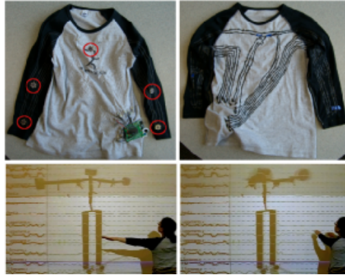
Figure 2.1: Motion capture system based on accelerometers. Adapted from [12].
