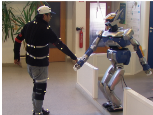
Figure 2.2: Motion capture system based on markers. Adapted from [13].
